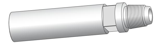
The check valve is placed directly behind the hammer and prevents dirty water from entering the hammer through the bit when idle.
