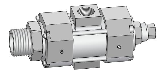
A swivel transfers the high-pressure water from the hose to the drill string. Wassara Swivels are designed and dimensioned to be robust and withstand the high pressure during water-powered drilling.
