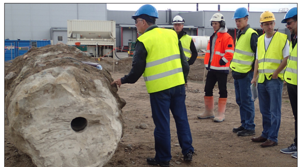
The Ø 120 cm test column
