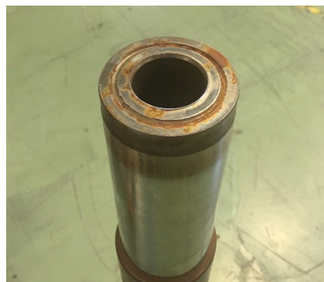
Piston after 2 500 meters of drilling
