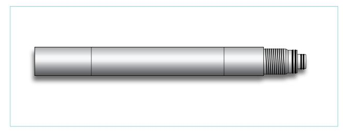
**Wassara Drill Tubes** are designed for maximum productivity optimal service life and to be easy to use. 4 seals are placed in the pin side of the tube to seal of any water and grout leakage. Material choices, heat treatments and production methods are all state of the art. Wassara duplex tubes have two channels with the inner designated for grout or any other substance (e.g. for precutting) and the outer designated for water used to power the hammer.
